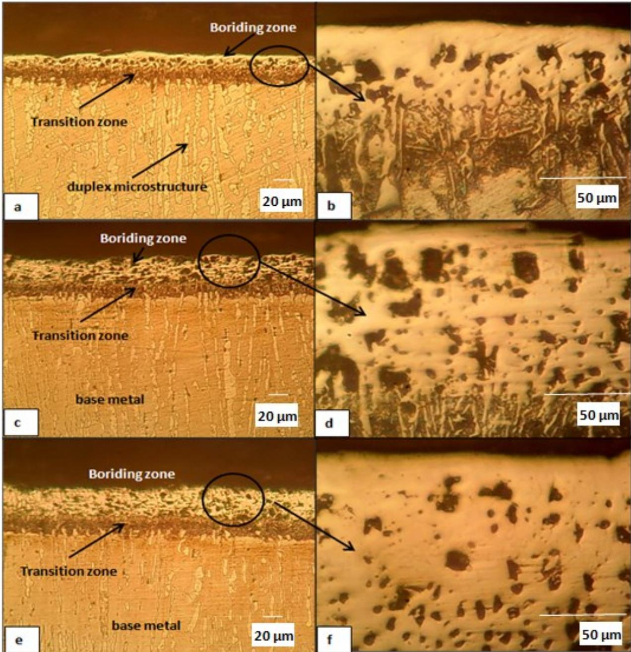
Figure 6. Optical microscopic images showing microstructure of duplex stainless steel UNS31803 exposed to boriding for: a, b) 2 h; c), d) 3 h; e, f) 4 h
