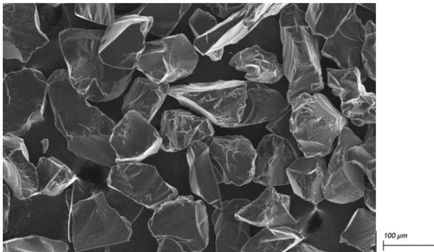
Figure 1. SEM image of the boriding medium
