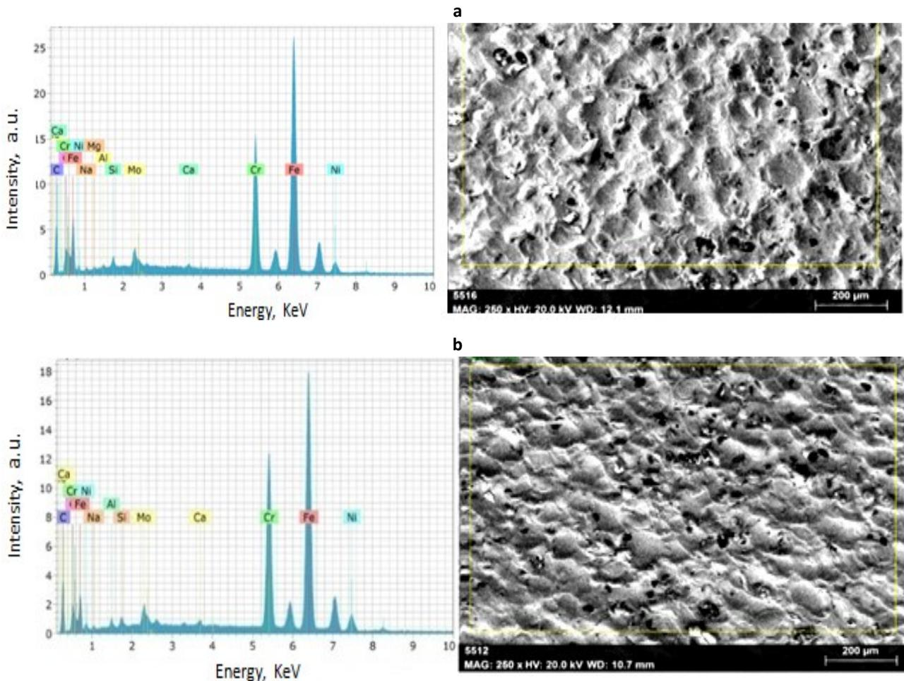
Figure 5. SEM micrographs and EDX analyses for materials exposed to the 4 h boriding process for: (a) duplex stainless steel UNS31803, (b) super duplex stainless steel UNS32750; (black dots in SEM micrographs correspond to surface pores; scale bar: 200 μm)
