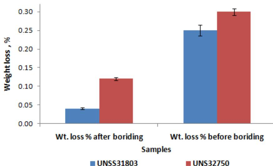
Figure 8. Weight loss comparison in the wear test
