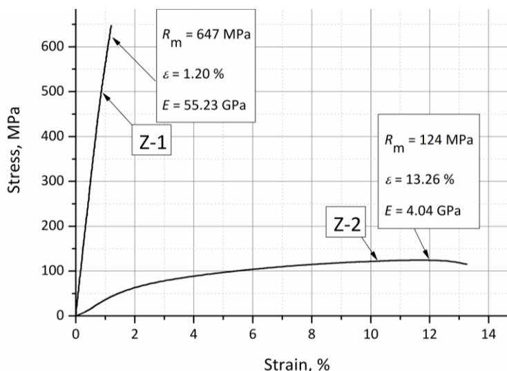
Figure 1. Typical comparative stress – strain curves for specimen series of  $0^\circ/90^\circ$  (Z-1) and  $\pm 45^\circ$  (Z-2) orientations with measured values of tensile strength ( $R_m$ ), strain ( $\epsilon$ ), and modulus of elasticity ( $E$ )
