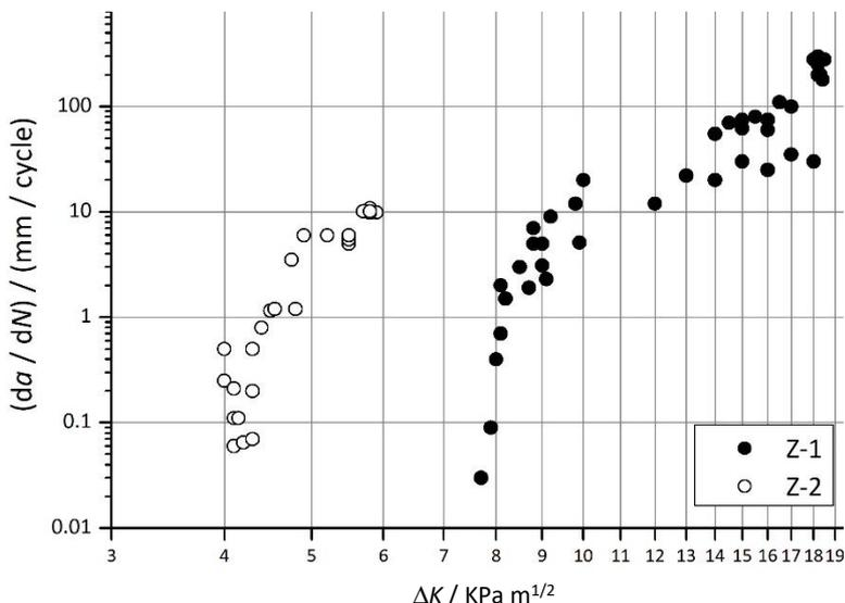
Figure 4. Measured constant-amplitude fatigue crack growth curves for Z-1 and Z-2 lay-ups
