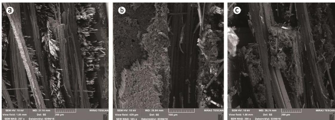
Figure 5. SEM micrograph of the fracture surface of the specimen Z-1: a) matrix cracking in 0° layers; b) delamination of the layers below the fracture surface; c) fiber delamination and a matrix crack
