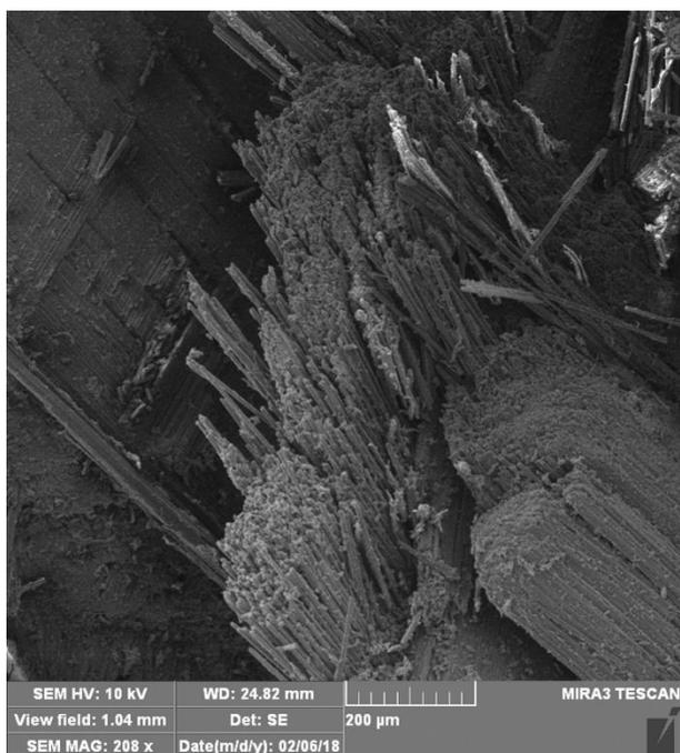
Figure 6. SEM micrograph of the fracture surface of the Z-2 specimen
