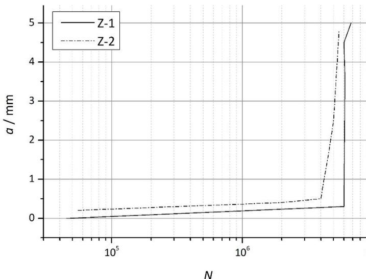
Figure 3. Fatigue crack growth: crack length, *a*, versus the number of cycles, *N*, for specimen series of 0°/90° (Z-1) and ±45° (Z-2) orientations
