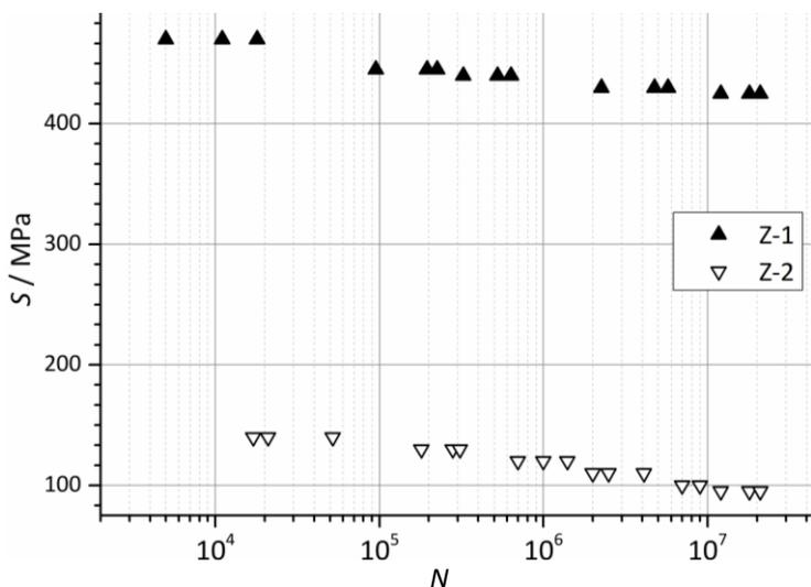
Figure 2. Comparative presentation of  $S-N$  curves for specimen series of  $0^\circ/90^\circ$  (Z-1) and  $\pm 45^\circ$  (Z-2) orientations
