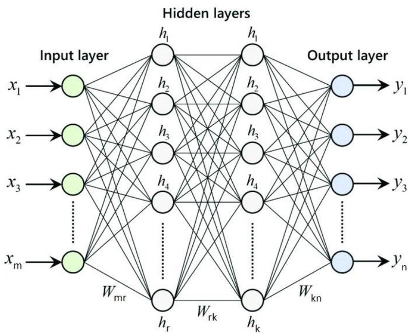
Figure 2. Multilayer perceptron architecture
