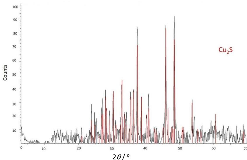
Figure 1. X-ray diffractogram for the chalcocite mineral
