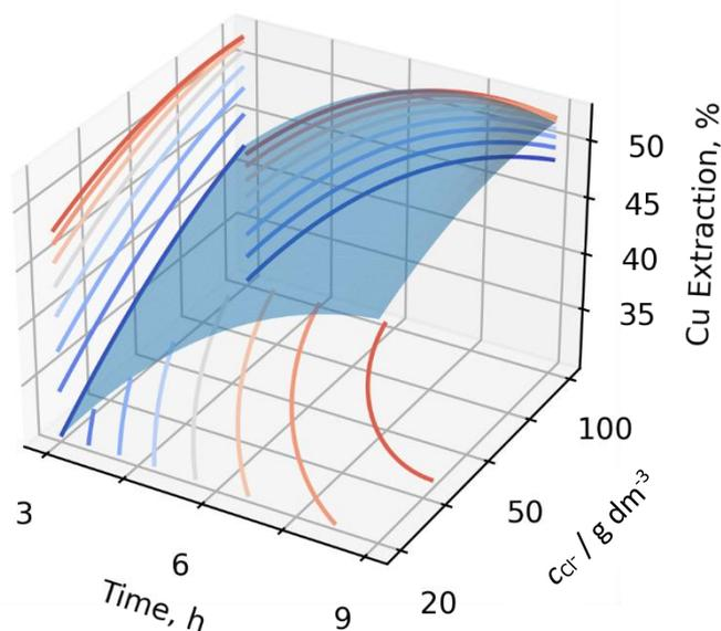
Figure 4. Response surface of the independent variables Cl concentration and time in copper extraction (plot generated matplotlib library in Python 3.7.0 programming language [52]).
