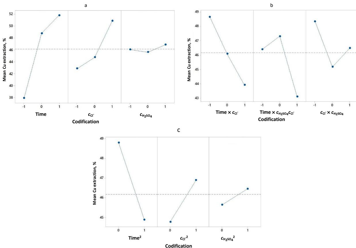
Figure 2. Plots of linear (a), interaction (b) and quadratic (c) effects of independent variables on copper extraction from chalcocite (plots generated in MINITAB 18 software[47])
