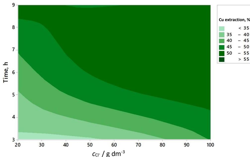
Figure 3. Contour plot of Cu extraction as a function of time and chloride concentration.
