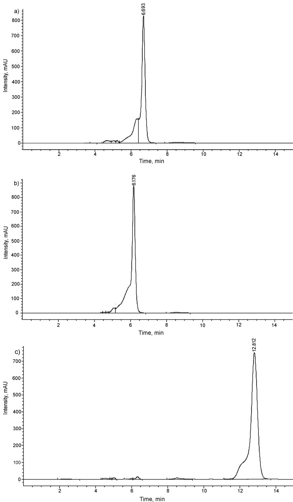
Figure 3. HPLC chromatograms of NIPMAM (a), NIPAM (b) and EGDM (c)
