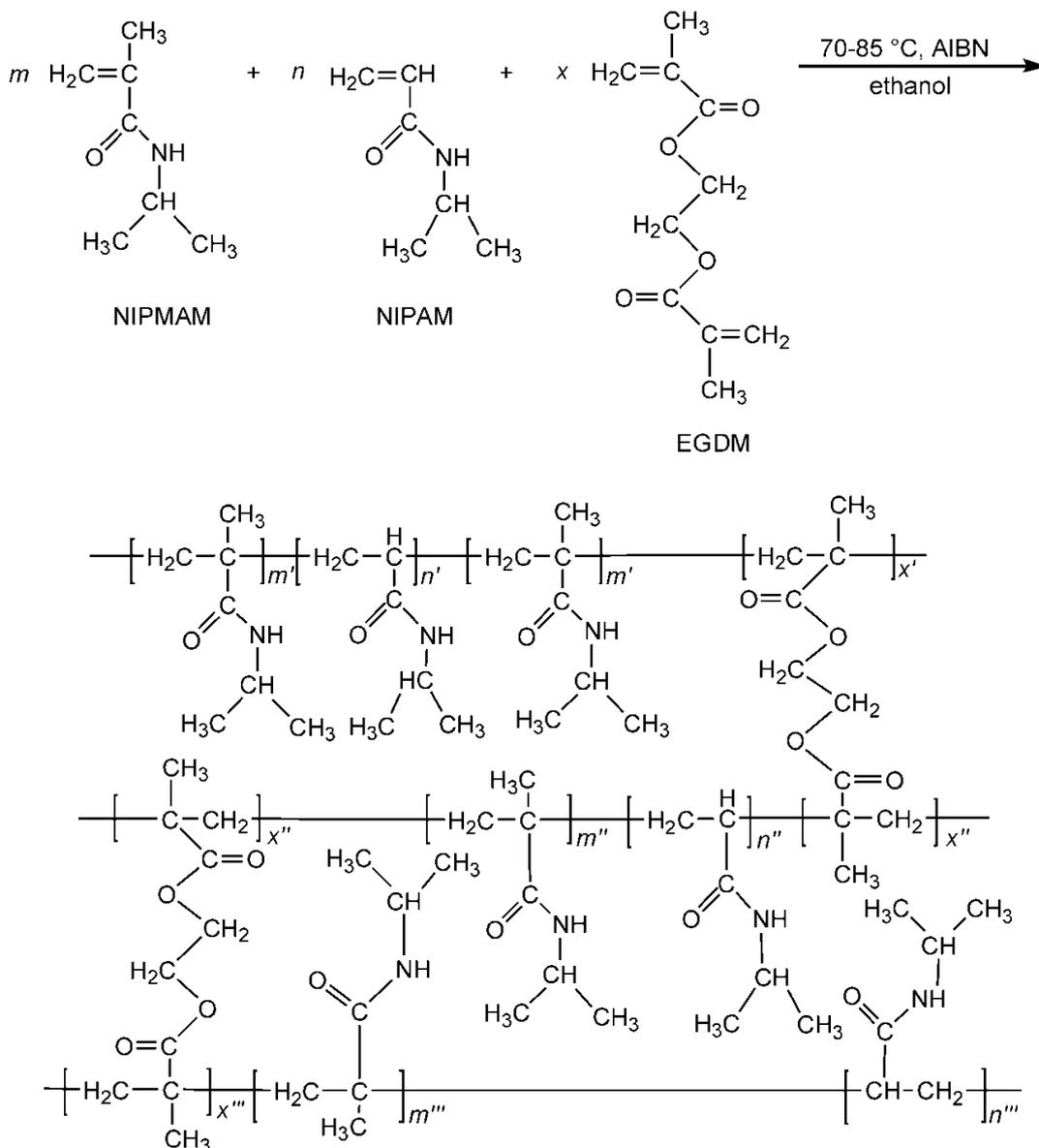
Figure 1. Schematic representation of the synthesis and a possible structure of p(NIPMAM/NIPAM) hydrogels
