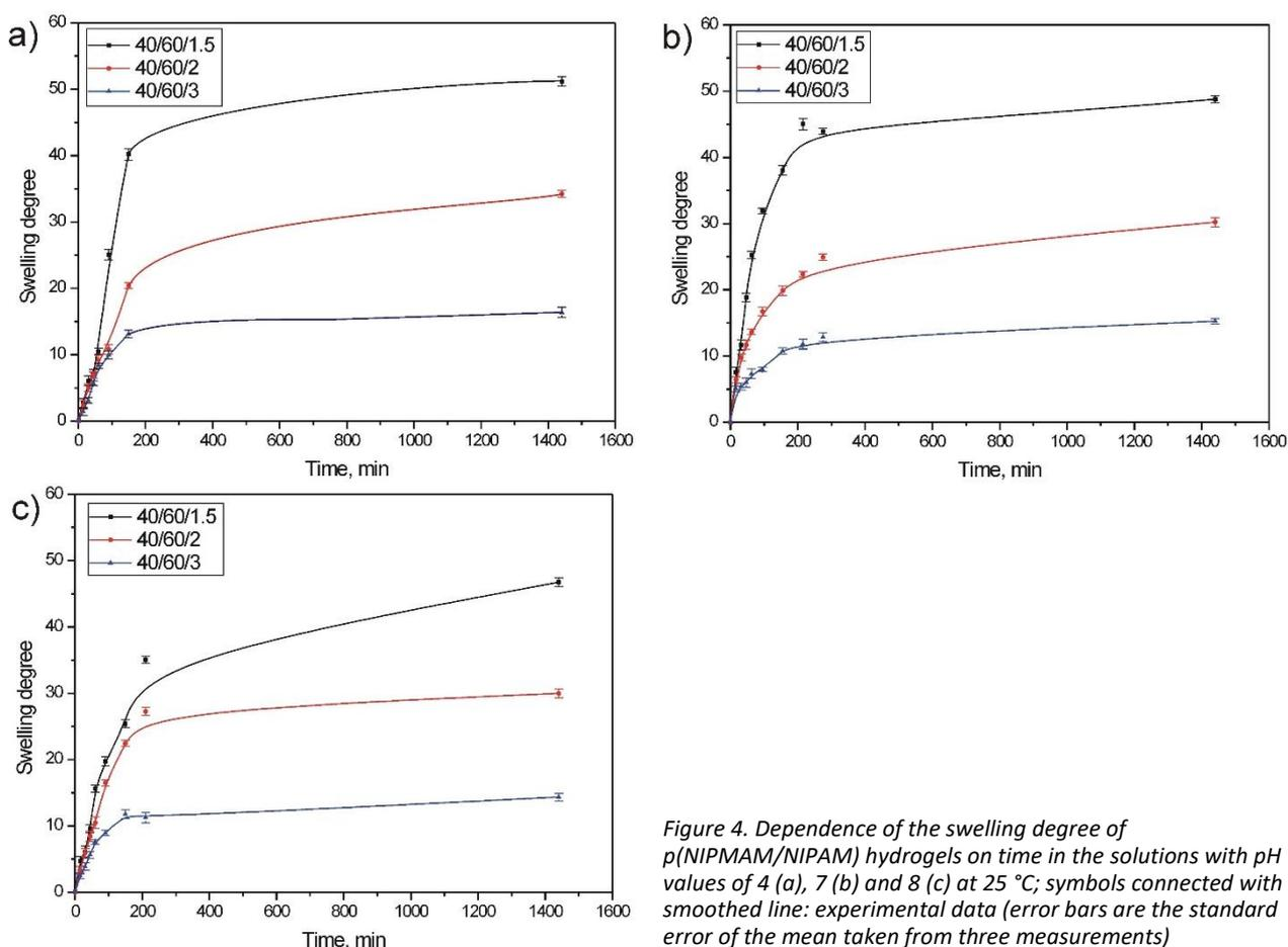
Figure 4. Dependence of the swelling degree of p(NIPMAM/NIPAM) hydrogels on time in the solutions with pH values of 4 (a), 7 (b) and 8 (c) at 25 °C; symbols connected with a smoothed line: experimental data (error bars are the standard error of the mean taken from three measurements)
