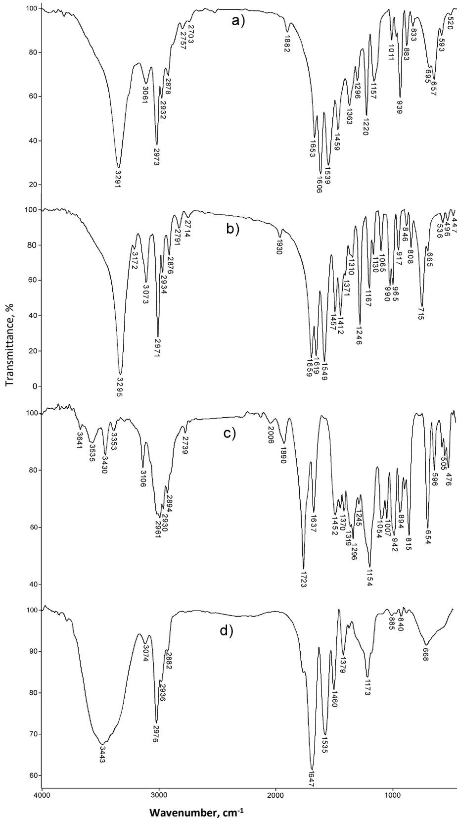
Figure 2. FTIR spectra of NIPAM (a), NIPAM (b), EGDM (c) and p(NIPAM/NIPAM) sample 40/60/3 (d)
