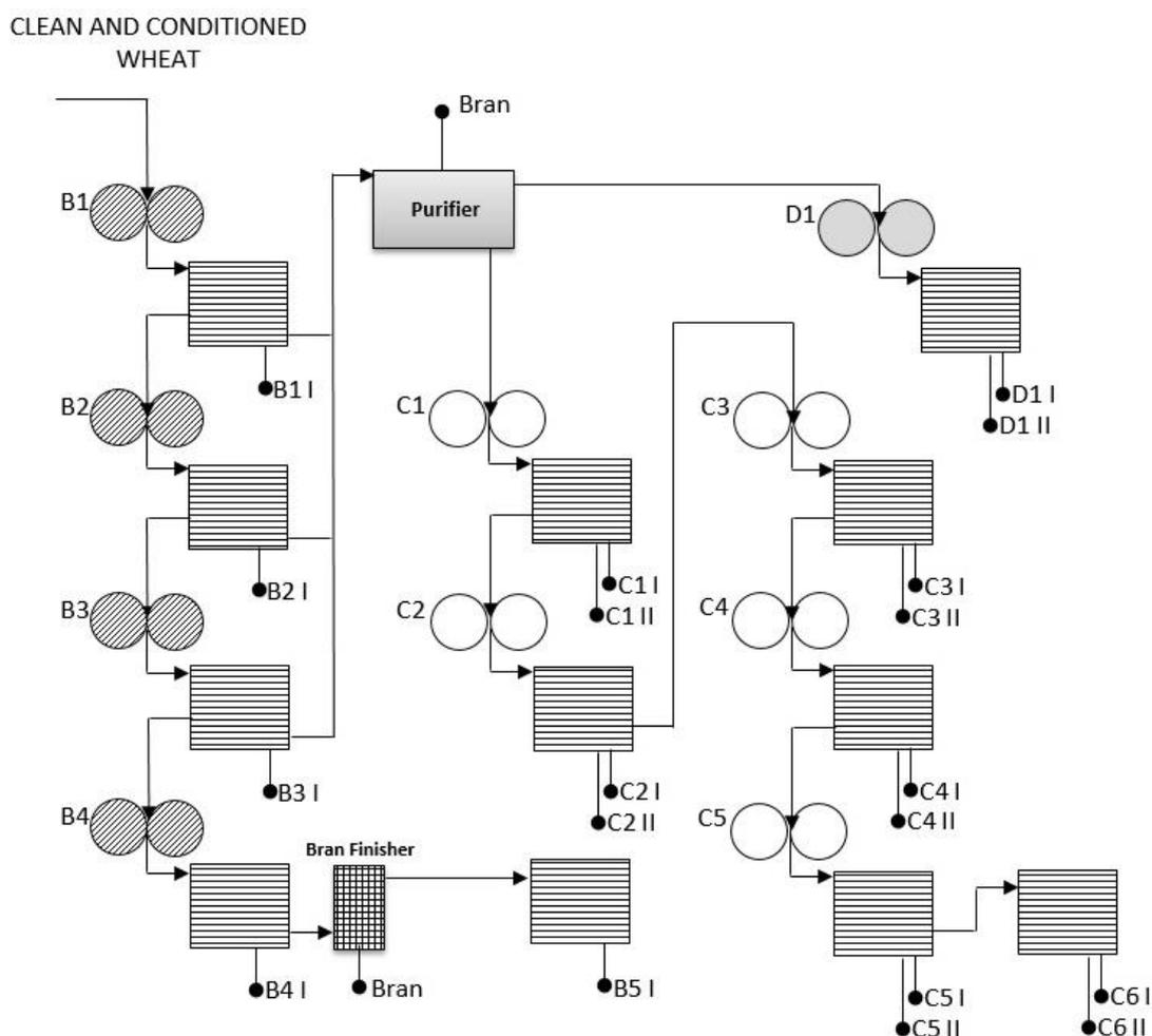
Figure 1. The simplified mill flow diagram. B1 I - B5 I: break flour streams; C1 I, C1II, C2 I, C2II, C3 I, C3II, C4 I, C4II, C5 I, C5II, C6 I, C6II: reduction flour streams; D1 I – D1II: purifying flour streams
