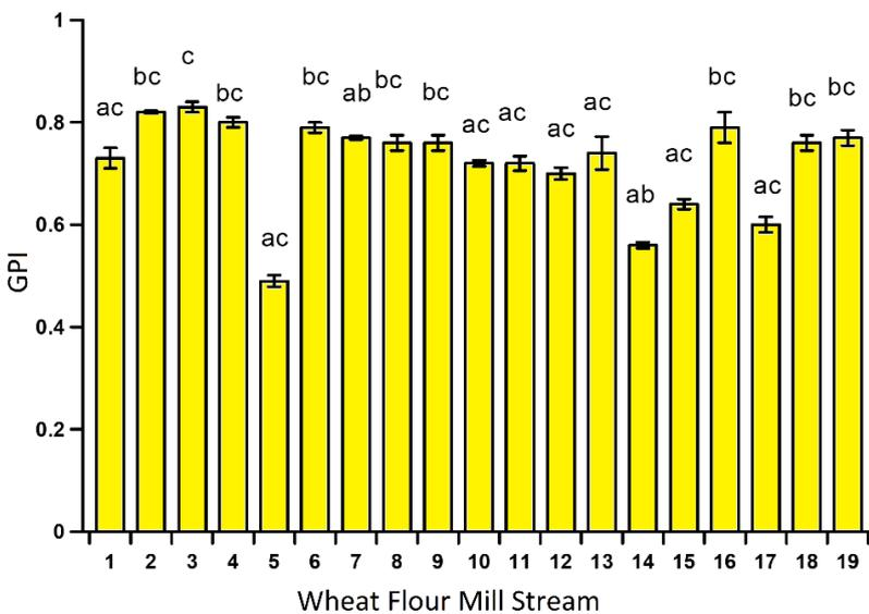
Figure 3. Glutenin performance index of wheat flour mill streams; 1-5: break flour streams; 6-17: reduction flour streams; 18-19: purifying flour streams. Different letters of bars denote significant differences (Tukey's test  $p > .05$ )
