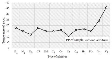
Fig. 4. PP as a function of different additives at the concentration of 1000 ppm for "fresh" rapeseed biodiesel (sample 2)
