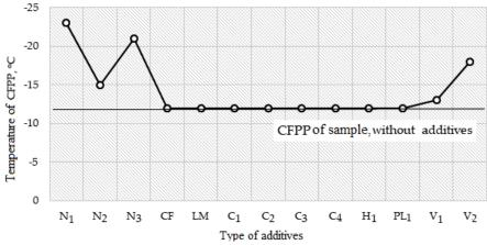
Fig. 5. CFPP as a function of different additives at the concentration of 1000 ppm for the mixture of BD-100 (rapeseed biodiesel) and ULSD (5:95) (sample 3)
