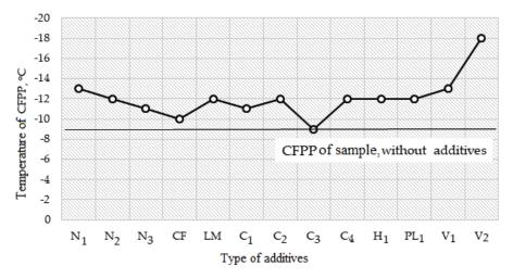
Fig. 3. CFPP as a function of different additives at the concentration of 1000 ppm for "fresh" rapeseed biodiesel (sample 2)
