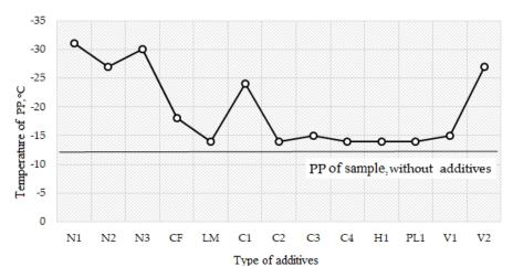
Fig. 6. PP as a function of different additives at the concentration of 1000 ppm for the mixture of BD-100 (rapeseed biodiesel) and ULSD (5:95) (sample 3)
