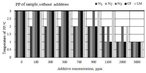
Fig. 2. PP vs. concentration of different additives, for "aged" biodiesel with palm oil (sample 1)
