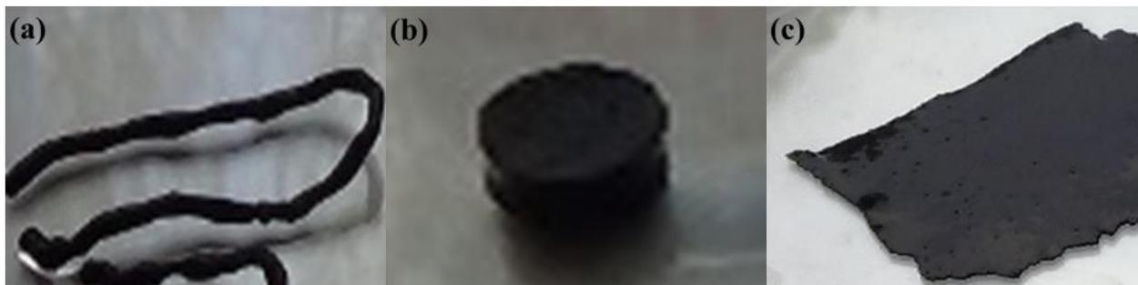
Figure 2S. Composite ZnA/AC hydrogel in the form of (a) fibre; (b) sheet; (c) film
