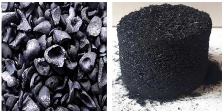
Figure 1. Carbonized apricot pits and AC after carbonization
