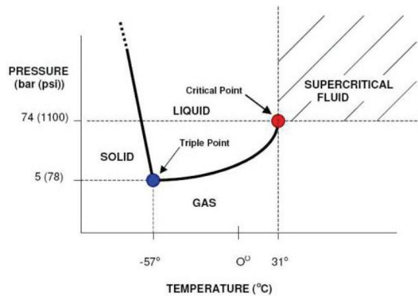
Figure 1. Phase diagram for CO<sub>2</sub>.
