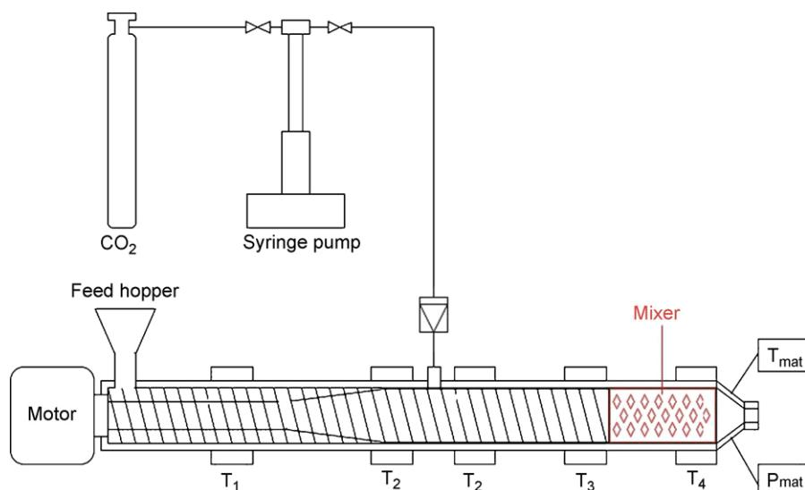
Figure 2. Shematic diagram of SCFX extruder [5].
