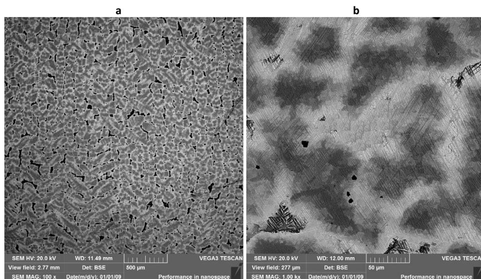
Figure 4. SEM image of the  $\text{Bi}_{18.6}\text{Sb}_{81.4}$  alloy, nominal magnification: (a) 100 $\times$  and (b) 1000 $\times$
