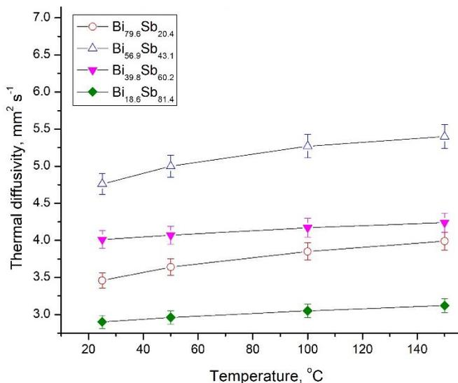
Figure 8. Temperature dependences of the experimentally determined thermal diffusivities of the examined Bi-Sb alloys (data are average of  $n=3$ )
