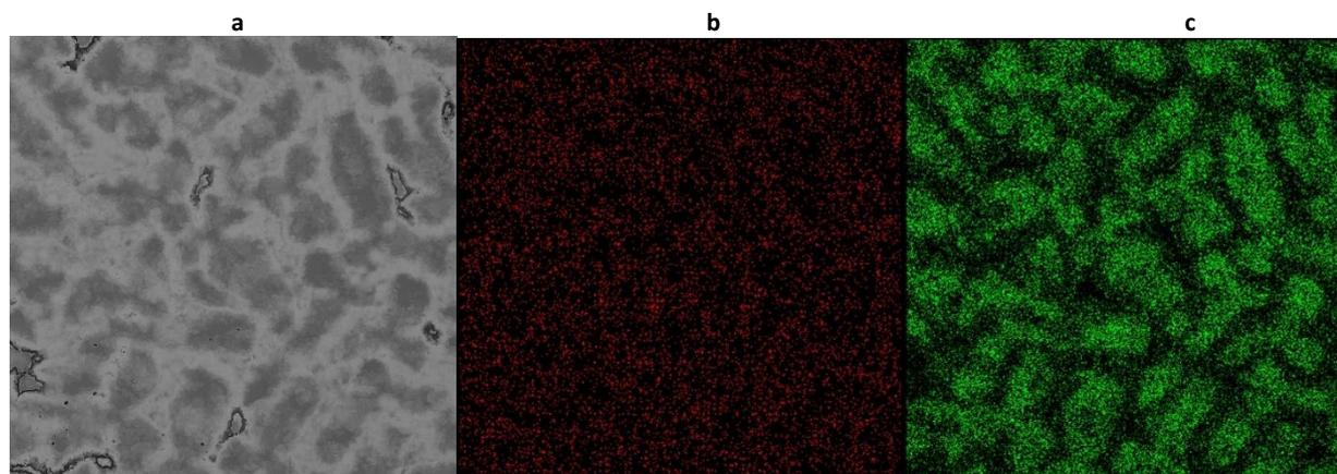
Figure 5. Elemental SEM-EDS mapping for the  $\text{Bi}_{56.9}\text{Sb}_{43.1}$  alloy: (a) microstructure, (b) Bi distribution, (c) Sb distribution (scale bar = 300  $\mu\text{m}$ )
