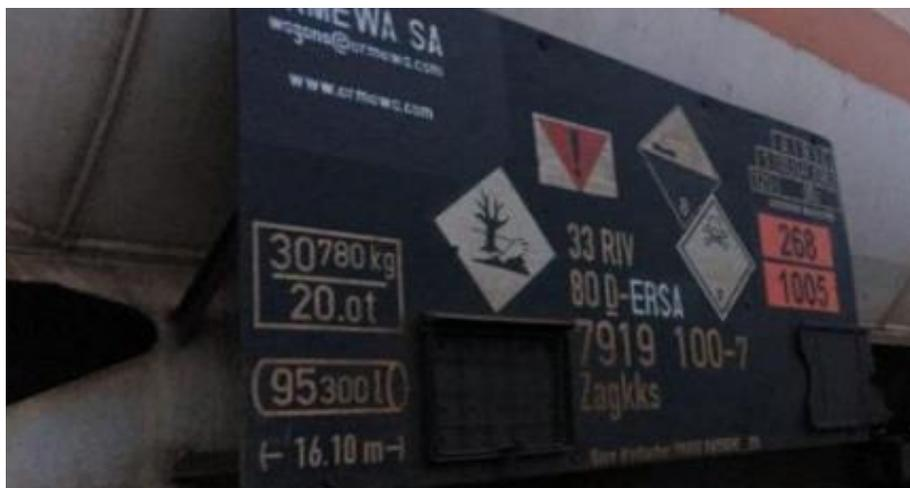
Figure 2. Specifications on tanks transporting ammonia
