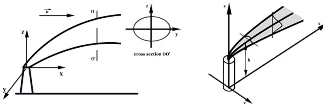
Figure 1. Orientation of the coordinate axes when modelling the smoke plume
