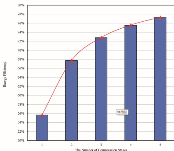
Figure 6. Exergy efficiency changes under different compression stages.
