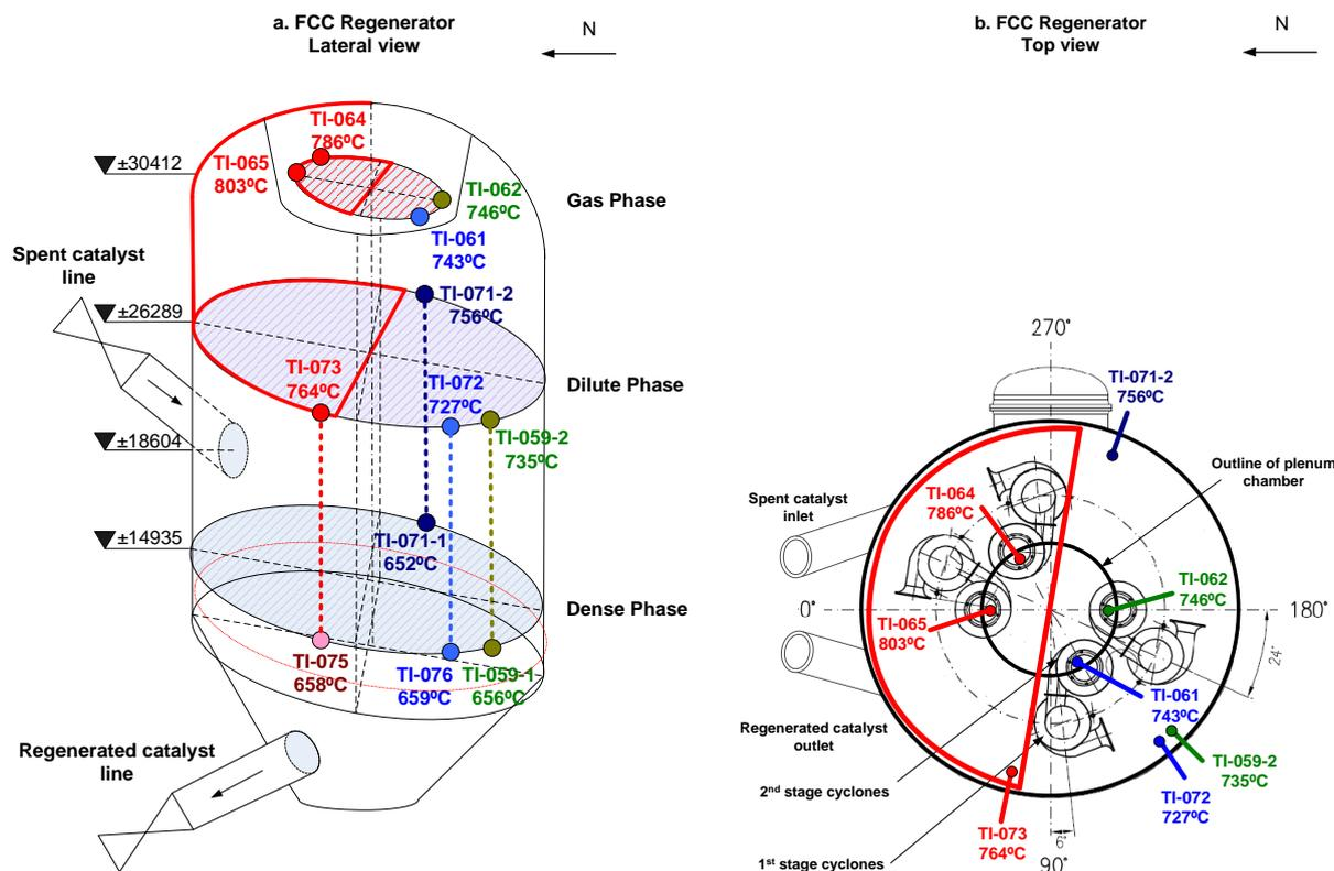
Figure 2. Temperatures registered by the regenerator's thermocouples on operation day no. 143: a. Regenerator lateral view - temperatures in dense, dilute, and gas phases; b. Regenerator top view - temperatures in dilute and gas phase.
