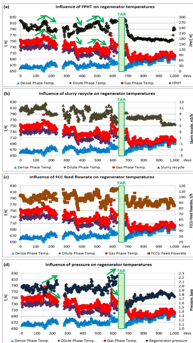
Figure 6. Influence of process parameters on regenerator temperature profile: a. Feed preheat temperature, b. Slurry recycle, c. FCC feed flow rate, d. Operating pressure.
