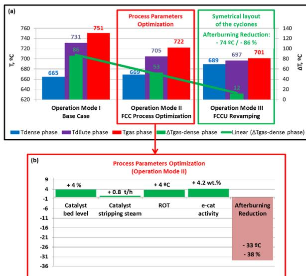
Figure 9. Afterburning reduction by FCC process optimization (a, b) and revamping (a).
