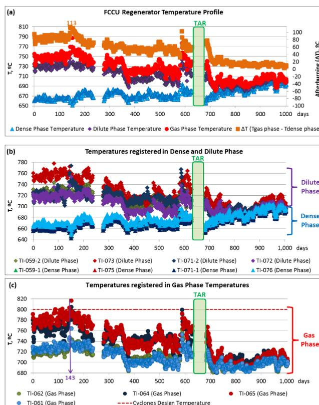
Figure 1. FCCU regenerator temperature profile: a. Average temperatures in dense, dilute, and gas phases; b. Temperatures registered by thermocouples in dense and dilute phases; c. Temperatures registered by thermocouples in the gas phase.
