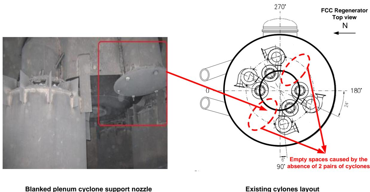
Figure 5. Non-symmetrical regenerator cyclones layout.
