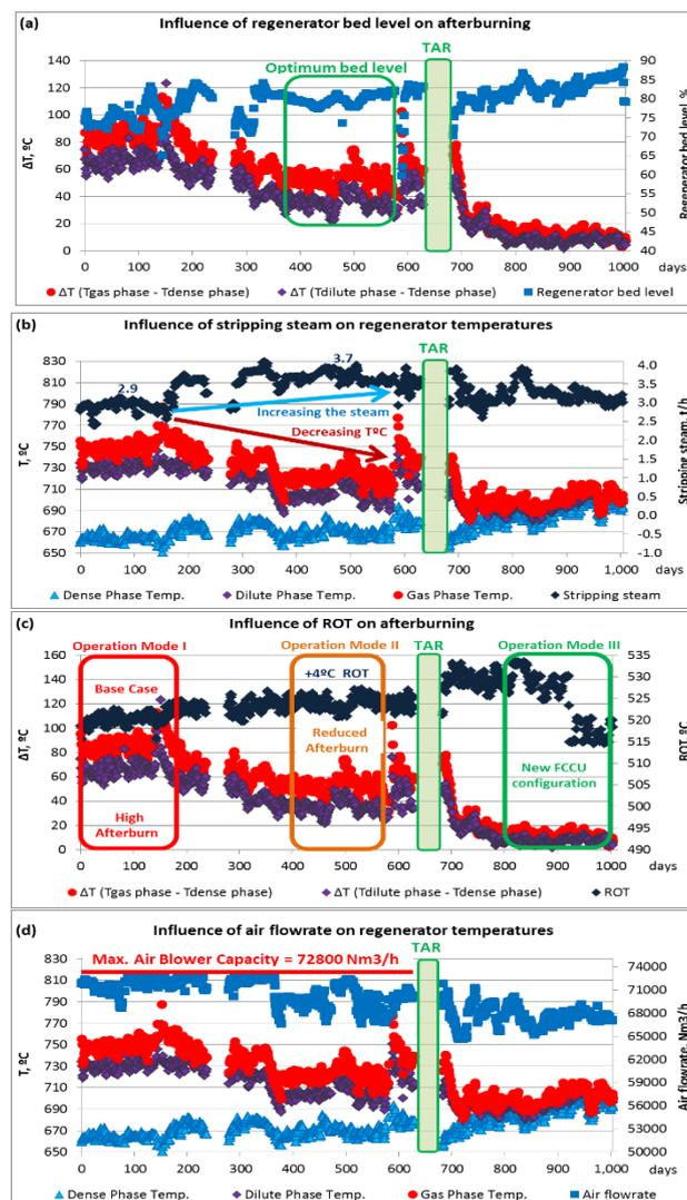
Figure 7. Influence of process parameters on regenerator temperatures: a. Regenerator bed level, b. Stripping steam, c. Riser temperature, d. Air flow rate.
