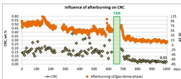
Figure 4. Increasing of CRC due to non-uniform mixing of air and catalyst.
