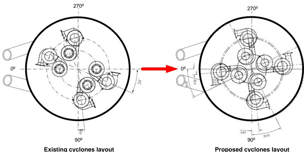
Figure 8. Replacing and assuring a symmetrical layout of the cyclones.
