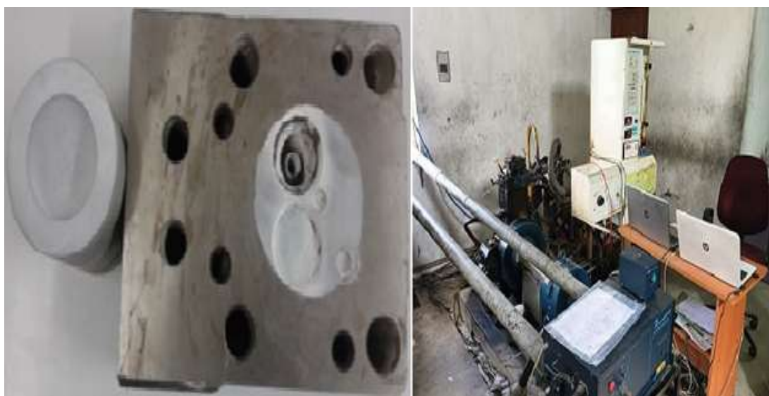
Figure 2 Nanocoated piston mounted in the cylinder head (left) and b) layout of test engine setup (right).
