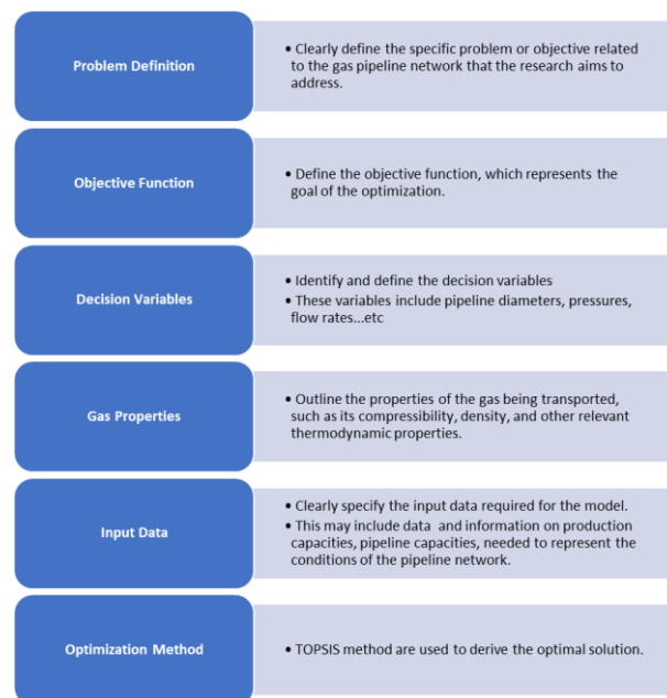
Figure 1. Flow chart of typical steps involved in the TOPSIS approach.
