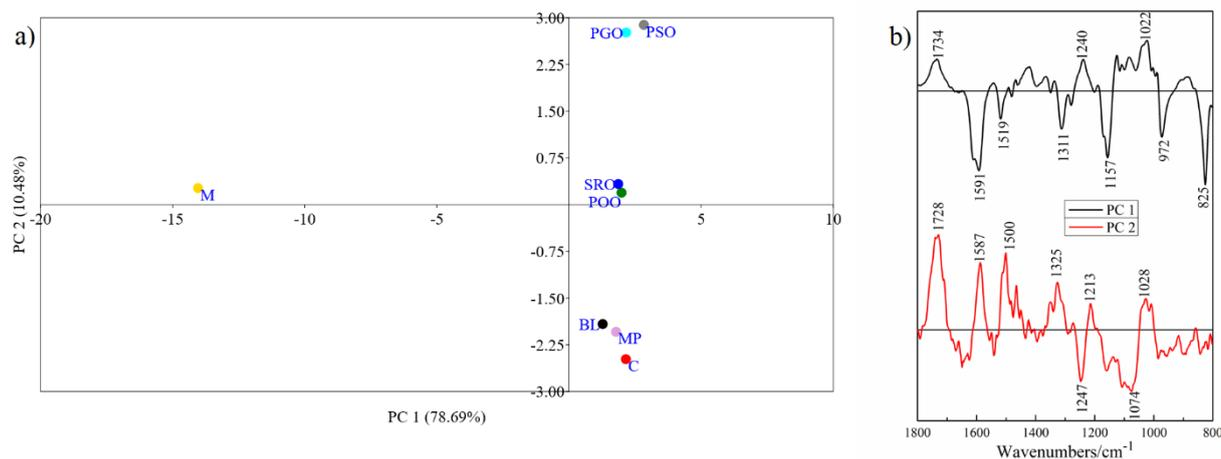
Figure 4. (a) Score plot of PCA for tested wood samples; (b) Loading plots of PC 1 and PC 2.
