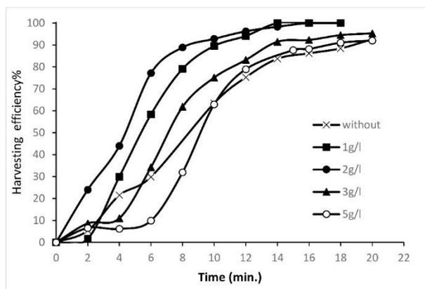
Figure 2. The effect of electrolyte concentration on the harvesting efficiency for the graphite anode.
