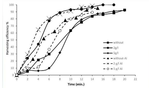
Figure 3. Comparison of graphite and aluminum anodes' harvesting efficiencies with different electrolyte concentrations. The solid line represents the graphite electrode, and the dashed line represents the aluminum electrode.
