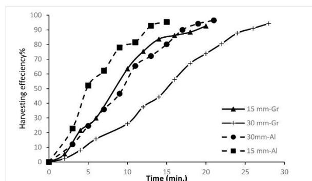
Figure 5. Harvesting efficiency of graphite and aluminum anodes with a distance between the electrodes of 15 mm and 30 mm. The solid line represents the graphite electrode, and the dashed line represents the aluminum electrode.
