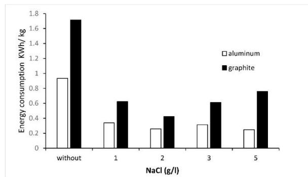
Figure 4. Comparison between the energy consumption of graphite and aluminum anodes with different electrolyte concentrations.
