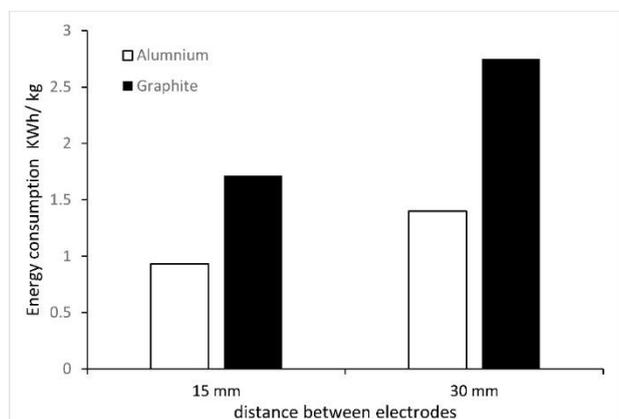
Figure 6. Effect of distance between electrodes on energy consumption for aluminum and graphite electrodes.
