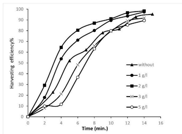
Figure 1. The effect of electrolyte concentration on the harvesting efficiency for the aluminum anode.
